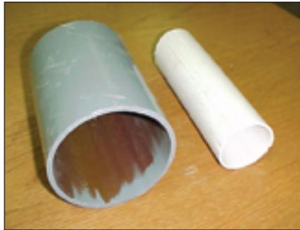
The biofilm-encrusted pipe sample (left) was disinfected by chlorine gas; the nearly spotless pipe (right) was exposed to mixed-oxidant treatment.
