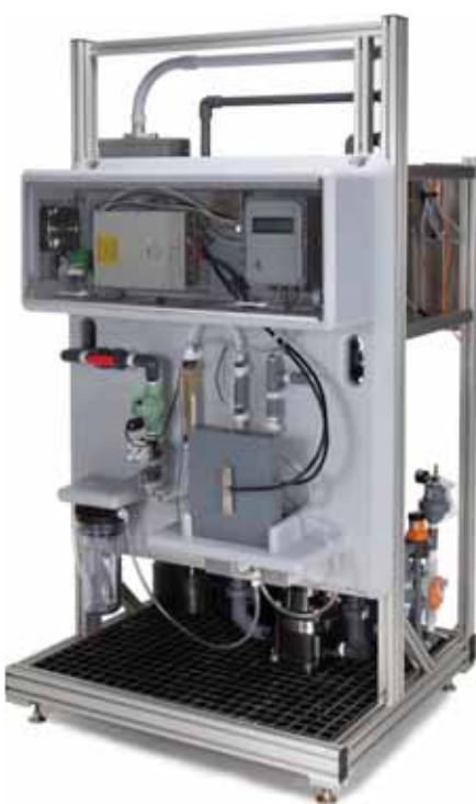
The onsite disinfection system produces a mixed-oxidant solution to reduce biofilm and algae.
