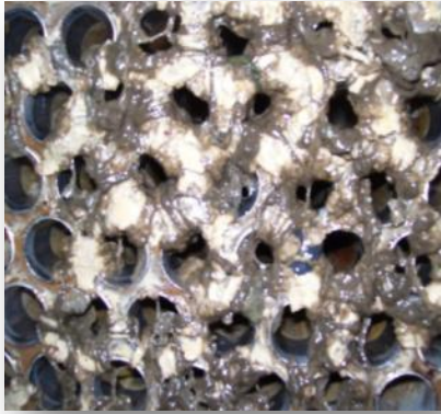
Condenser Tube Sheet BEFORE MOS
