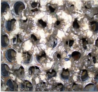
Condenser Tube Sheet BEFORE MOS
