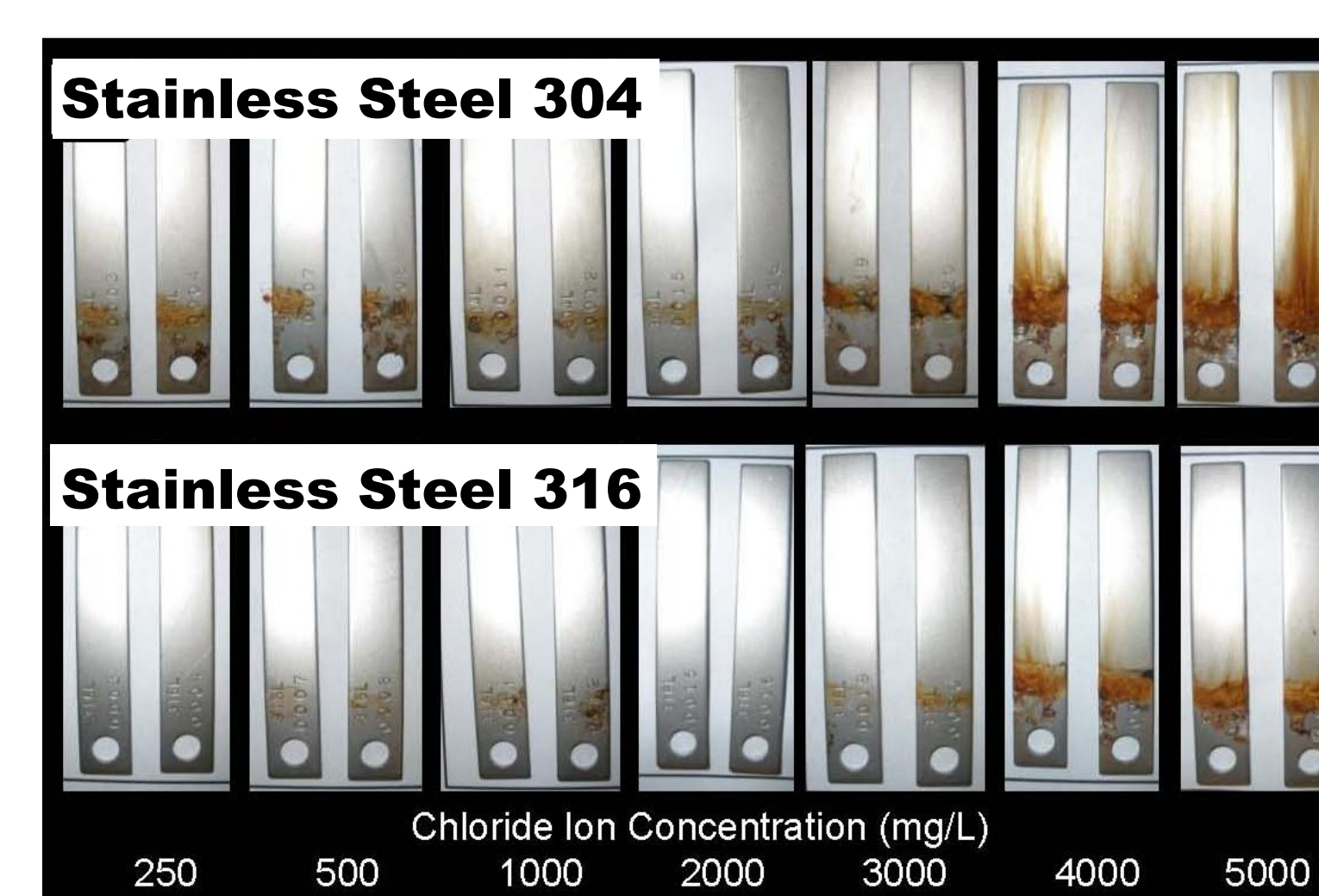
Photographs of coupons exposed to variable chloride ion content bleach for six weeks
